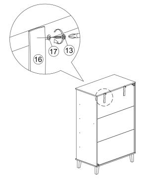
4. Add safety strap (16), washer (17) using 3.5x15mm screw (13) to back of cabinet.
