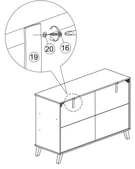
4. Add safety strap (19), washer (20) using 3.5x15mm screw (16) to back of cabinet.
