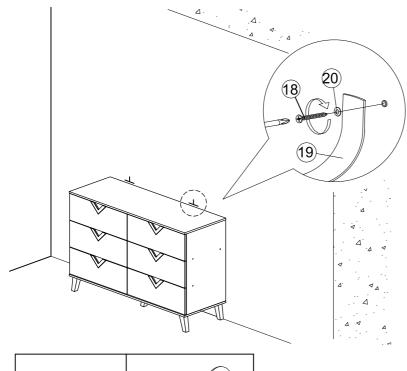
5. Finally, attach safety strap (19) and washer (20) using 4x30mm screw (18) to the wall.
